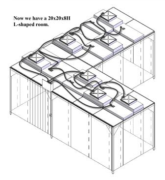
Once again we were able to use the curtains from one wall of the original 8x8x8H room on the end of the new addition. Also we were able to add the filters and lights to the existing Prefab Wiring Kit.
