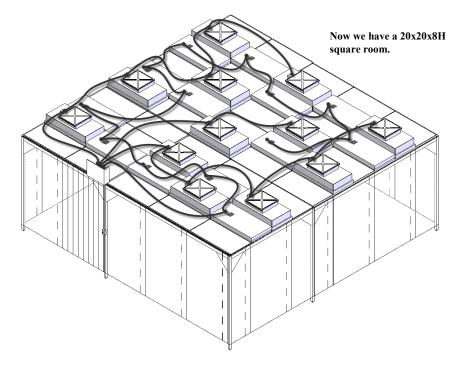
Once again we were able to use curtains from the existing room additions on the ends of the new addition. Also we were able to add the filters and lights to the existing Prefab Wiring Kit. The NCI SWCR can expand as you do.
