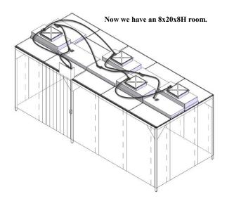
Note that we were able to use the curtains from one wall of the original 8x8x8H room on the end of the new addition. Also we were able to add the filters and lights to the existing Prefab Wiring Kit.
